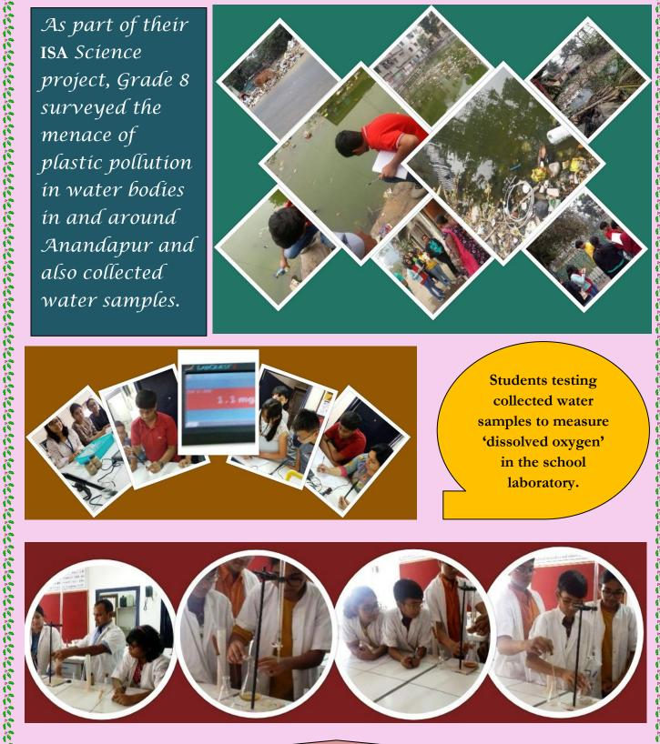
Iodometry titration done by students using the collected sample of water to calculate BOD (Biological Oxygen Demand).
